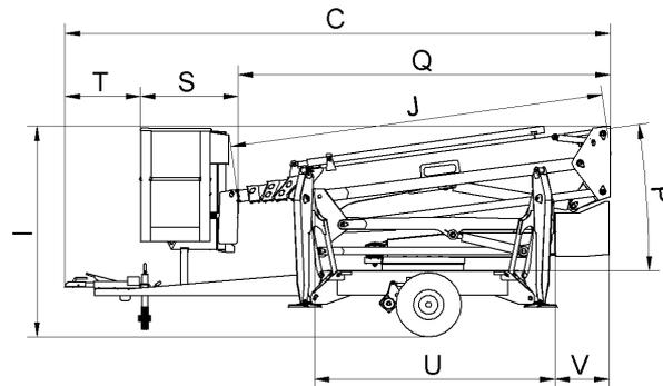
**Figure 2 Telescopic work platform in transport position**
