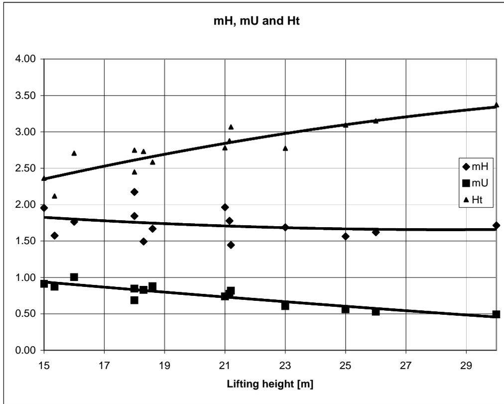
Figure 4 Values mH, mU and Ht of 15 investigated telescopic work platforms
