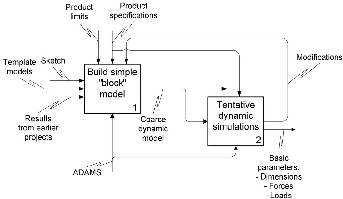
**Figure 5. Conceptual simulation phase (A41).**
