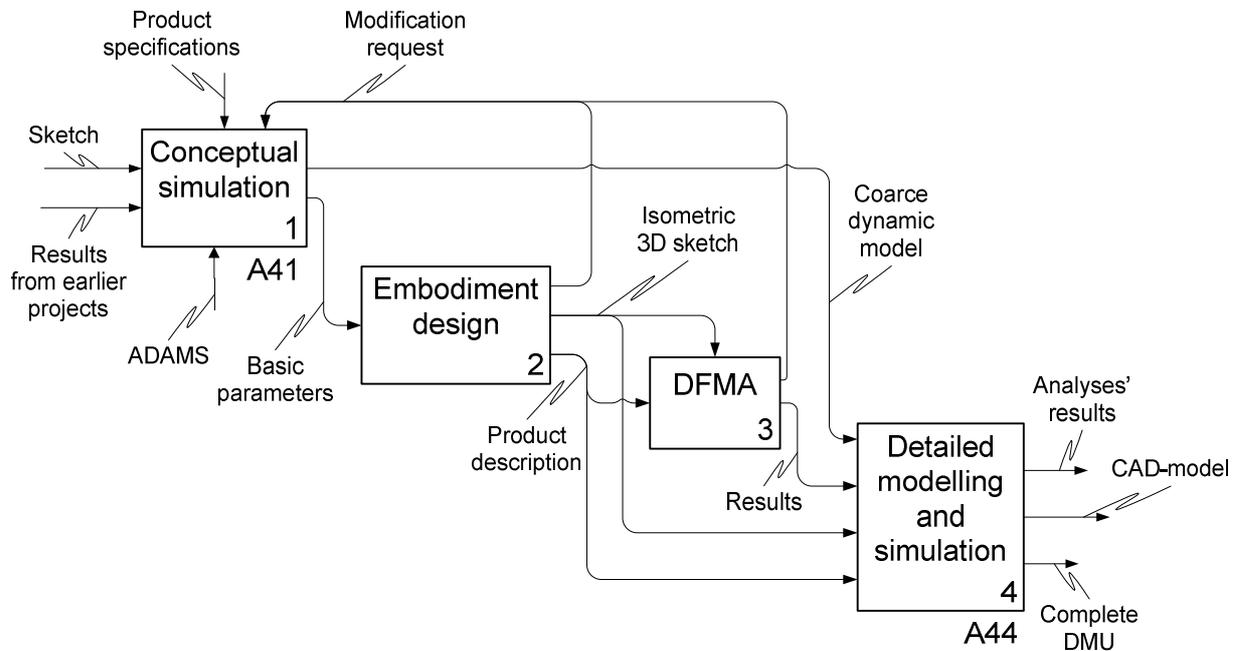
**Figure 4. Product modelling phase and the information flow in it. (A4)**
