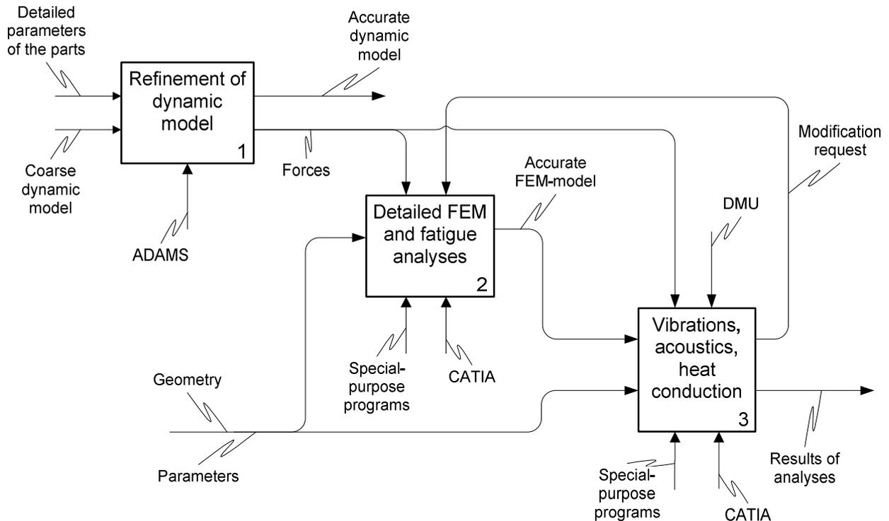
Figure 7. Detailed simulation and analyses. (A442)
