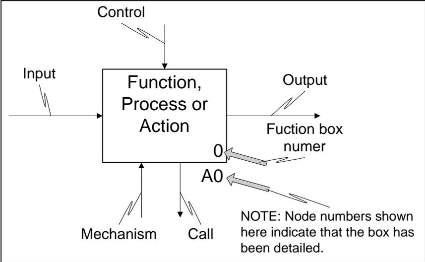
Figure 1. The basic function of IDEF0 activity box
