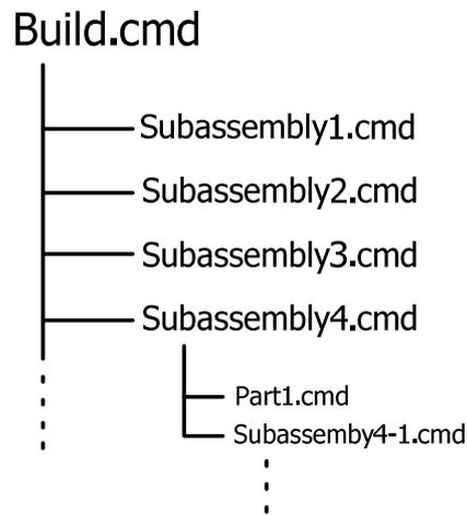
Figure 3. A tree structure constituted using ADAMS command file
