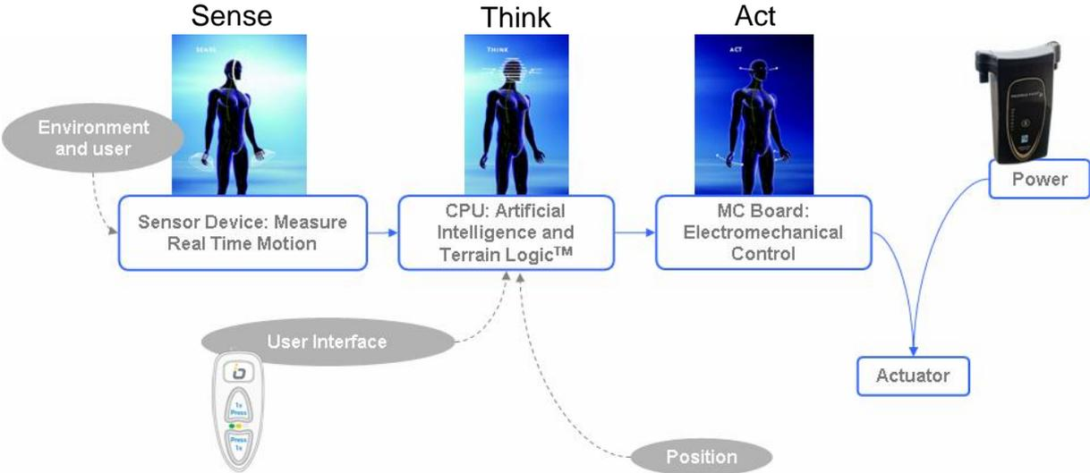
**Picture 2. High Level Technical Architecture of a microprocessor controlled prosthetic foot**
