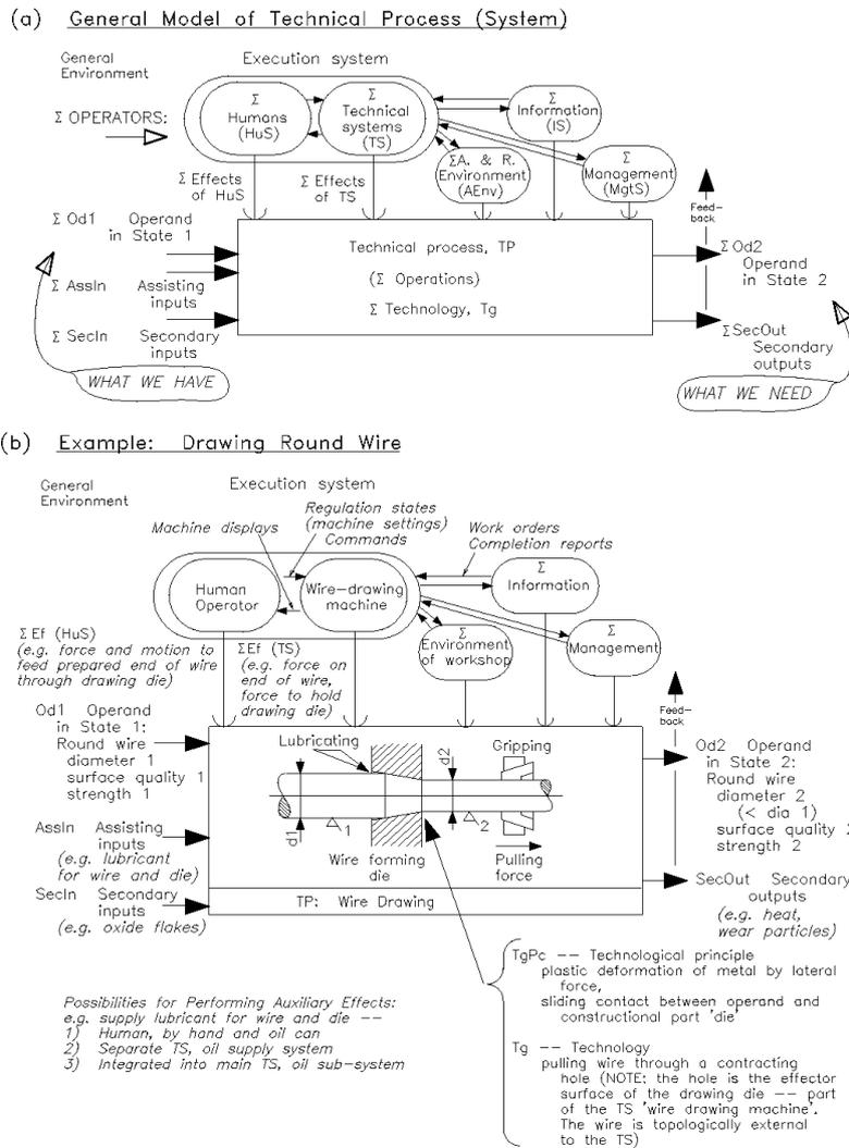
Figure 4. Example: Wire Drawing
