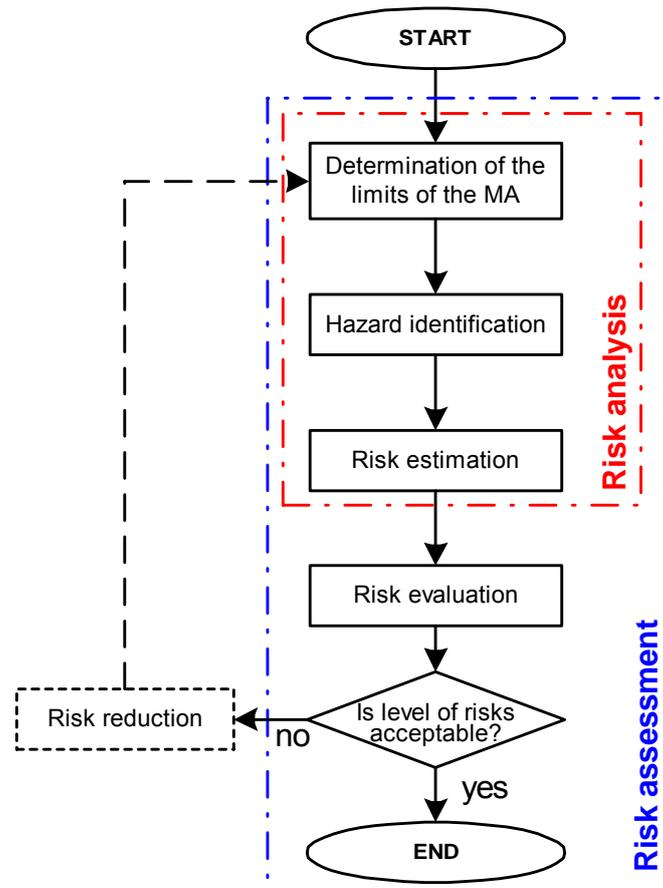
**Figure 3. Repeated procedure to ensure machinery safety in accordance with EN 1050**
