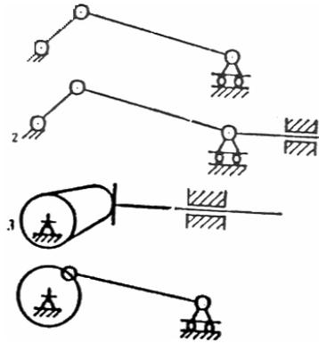
**Figure 3. Some principles realizing the transformation of the continue rotating motion into alternative translation motion.**
