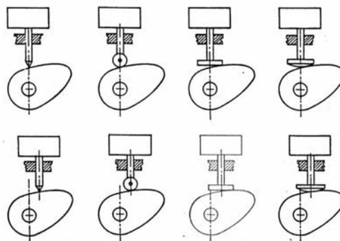
**Figure 4. Principles with return of the moved member by weight**
