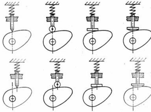
**Figure 5. Principles with return of the moved member by spring.**
