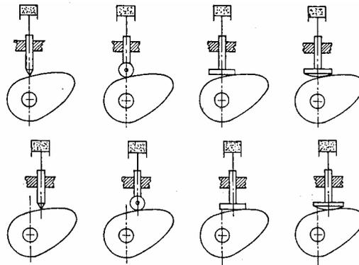
**Figure 6. Principles with return of the moved member by gas pressure.**
