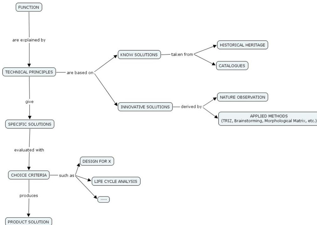
**Figure 1. Concept maps scheme of the method to identify the technical principles that perform functions.**
