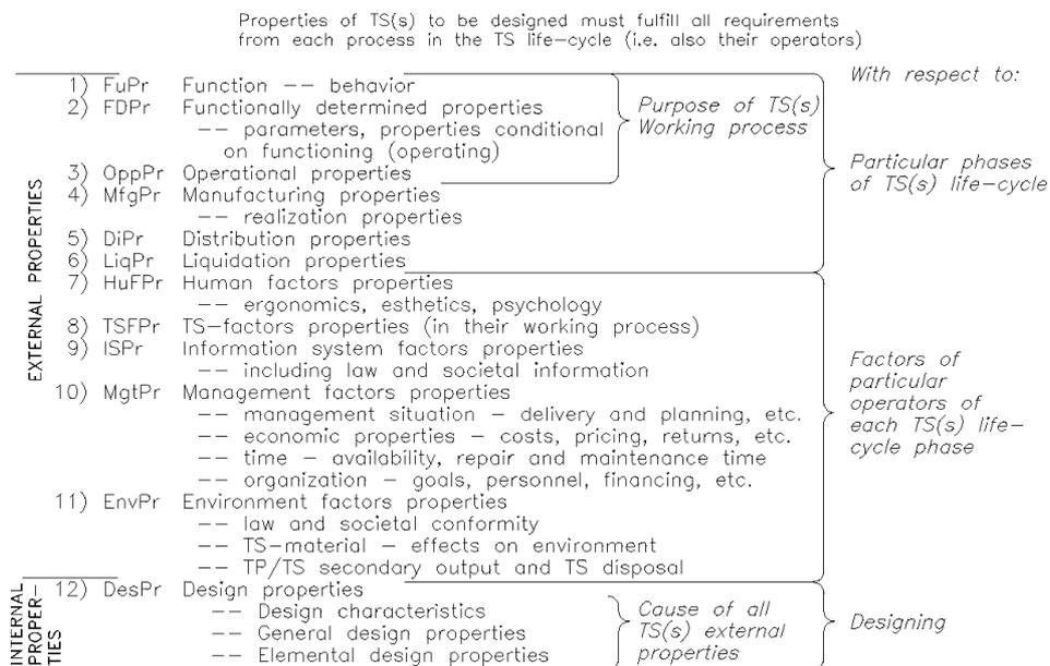
Figure 2 Classes of Properties of Technical Systems
