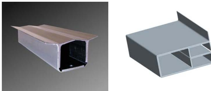
Figure 5: Possible Profile Structures made by Linear flow Splitting
