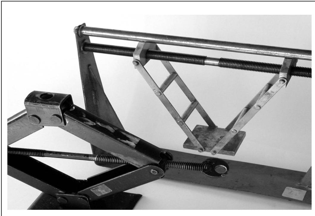
Figure 4. The proprietary scissor jack used as a source of ideas
