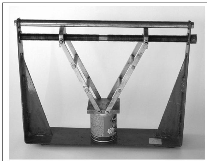
Figure 3. A student engineer's can crusher
