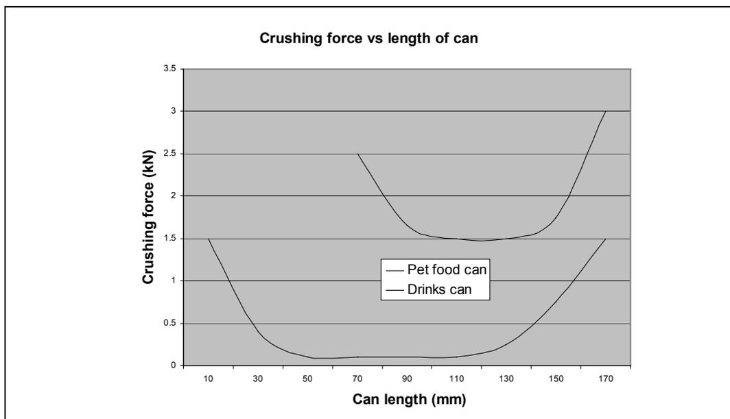
Figure 1. Task characteristic for axial crushing of steel cans
