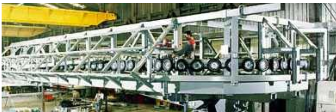
Figure 1. A beam of wheels under assembly
