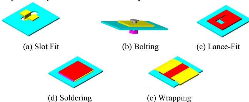
Figure 7 Form of different PDEs/solutions for “*Semi-Permanent Assembly*” function
