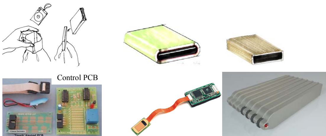
Figure 3. The Pandora Box. The Pandora's box has a rather aggressive look with diodes on each side to signal that the alarm is on. Fingerprint scanner for identification.
