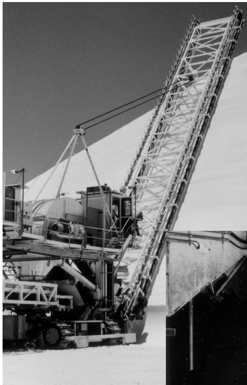
Figure 1. Salt Reclaimer (inset shows cutting teeth)
