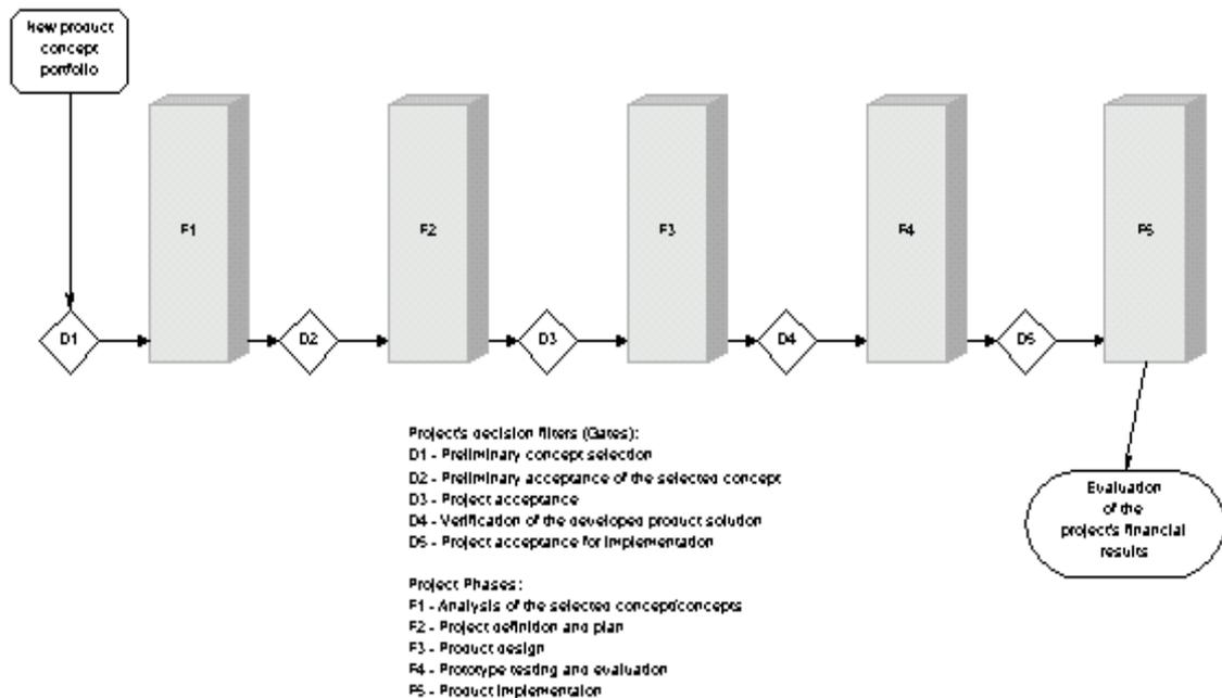
Fig. 3. Typical structure of the proposed Fast Product Development Process.
